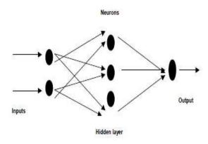
Figure 6: An Example of Single Output Neural Network, [25]
